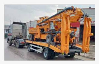
The frame of the FT 208 Trailer can be folded down while being shipped. For overseas shipments, the Scorpion Pump and its carrier trailer can be shipped with the same 40' HC container.
